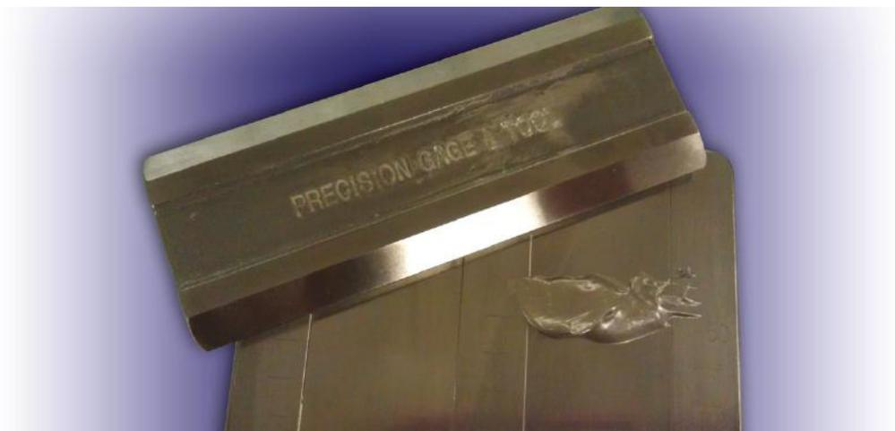
The resultant thin coating or film on the block is then visually inspected for any lumps or non-uniformities on the surface of the coating. Any visual observations can also be read using the scale along either side of the block. This scale can be read in Hegman units (dimensionless), micrometers or mils.
